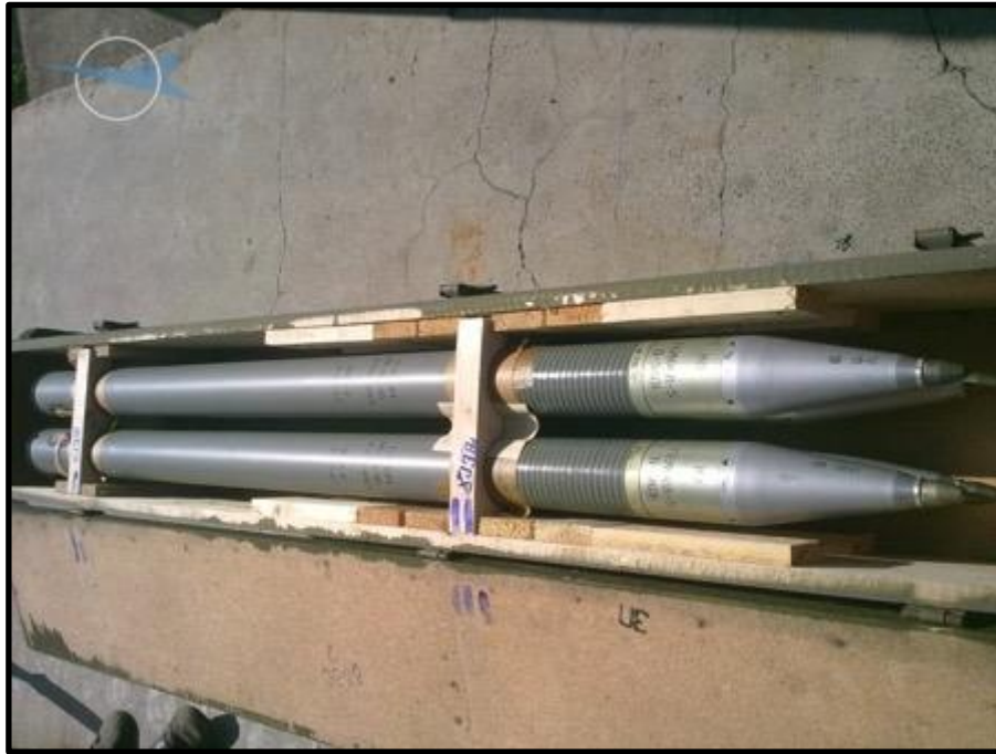
Figure 18: Screenshot from Khan Asparuh Trade showing the packing formation for S-8 KOM rockets
